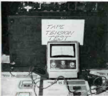
Minnetech Labs, Inc. (Nortronics). They manufacture instruments for the measurement of tension. The illustration shows a model designed to measure exact tape tension. The unit operates on a self-contained nicad battery or a.c. Versions are available with full-scale deflections as low as one ounce. Price: $325.00 without transducer. Circle 86 on Reader Service Card.
