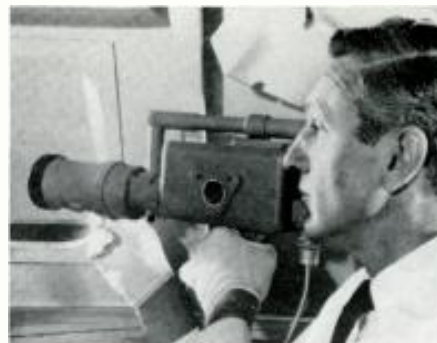
Figure 1. This four-and-a-half pound television camera is only 1/85th as large as those used in broadcast television studios. Such a camera-lens-viewfinder system was used on the Apollo 8 mission. Note in this official NASA photograph that the RCA logo has been obliterated.
