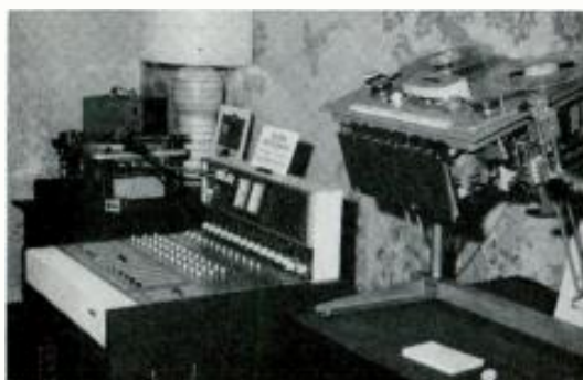
Gotham Audio Corporation. Gotham distributes Studer professional products. The console contains 12 inputs and a two-channel output. There is full equalization filtering, echo feed, pan pot for all channels, 20-watt stereo monitoring, peak-level metering, and two reverb channels. At right, is one of the Studer tape units. Circle 75 on Reader Service Card.
